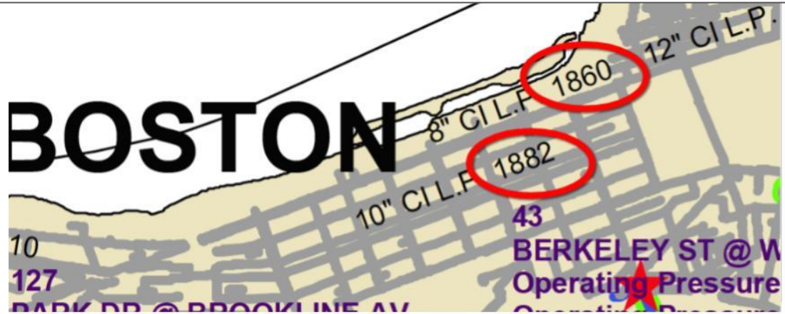
Detail of a National Grid gas infrastructure map of Back Bay showing two pipes from the 1800s still in use running down Beacon St and Comm. Ave.
